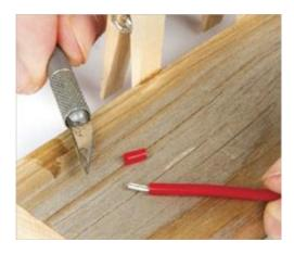
**1** Start by stripping the plastic insulation off the ends of the wires (usually, 3/16- to 1/2-inch is plenty).
