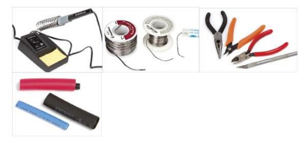
For basic wire, motor terminal and speed control soldering, you'll need:
