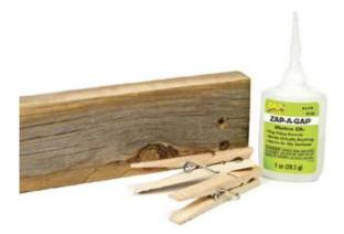
A piece of pine, two wooden clothespins and some ZAP is all that's needed to make a holding jig for soldering.
