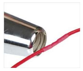
**5** Once the solder joint has cooled, slide the heat-shrink tubing over the joint and shrink it into place. I like to do this with a hot air gun used for shrinking plastic covering. It's quick and easy and the heat gun won't melt the wires or the solder.
